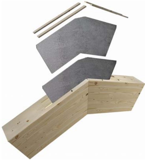
Figure 9: Example of a CNP joint with sheet inserts. The surfaces cannot be as smooth as they were originally, however they are revived with SA3 grade sandblasting and immediately protected with Xepox14 adhesive, applied by painting brush or roll.
